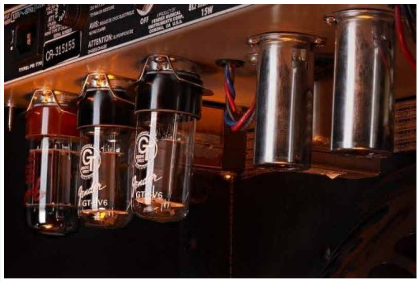
Figure 2: Internal view of the amplifier, highlighting the vacuum tubes which are crucial for its tonal characteristics.
