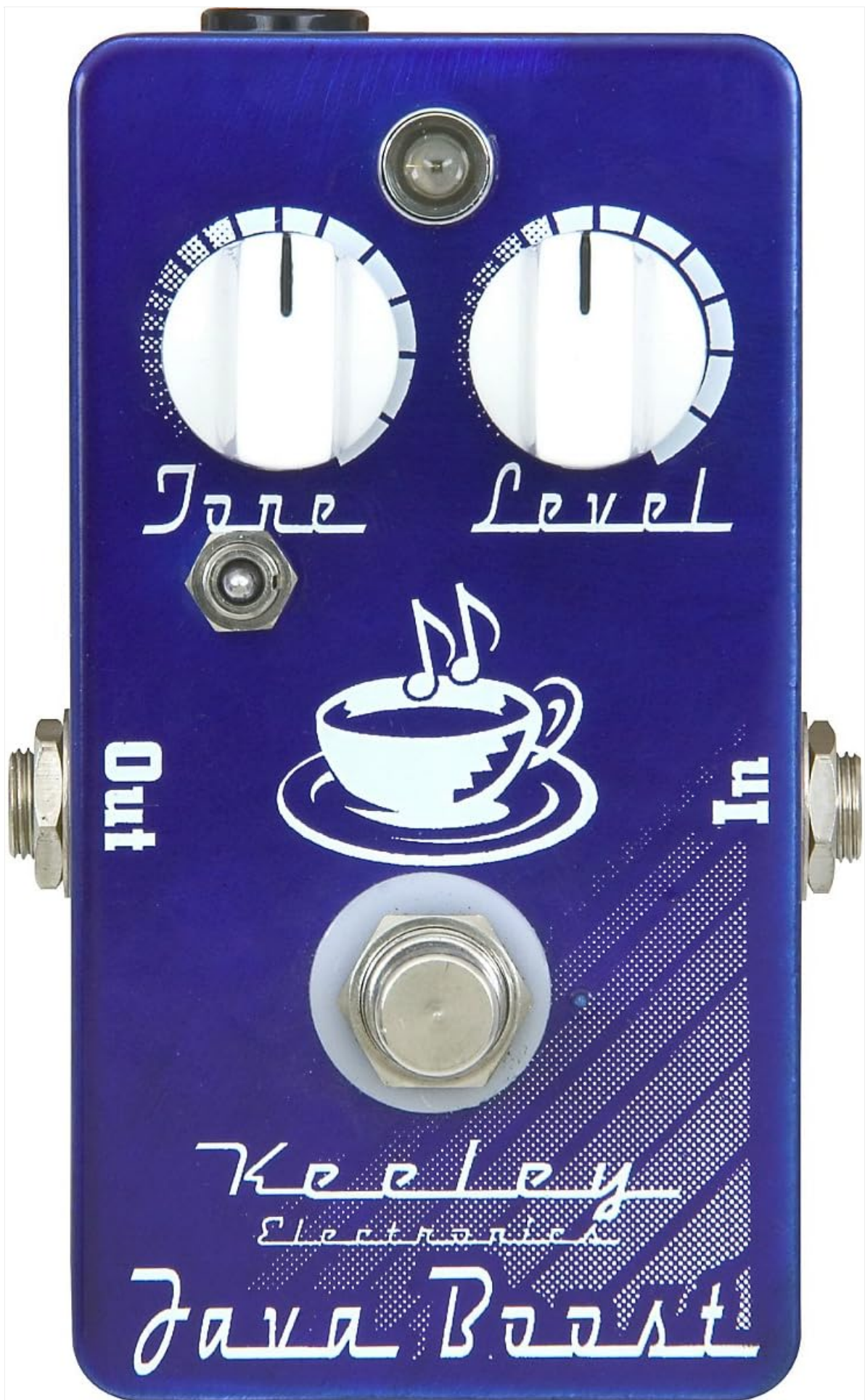
Figure 1: Front view of the Keeley Java Boost pedal. This image displays the pedal's top panel, highlighting the 'Tone' and 'Level' control knobs, the 'In' and 'Out' jacks on the sides, and the central footswitch. The pedal is a vibrant blue with white text and graphics, including a coffee cup logo.
