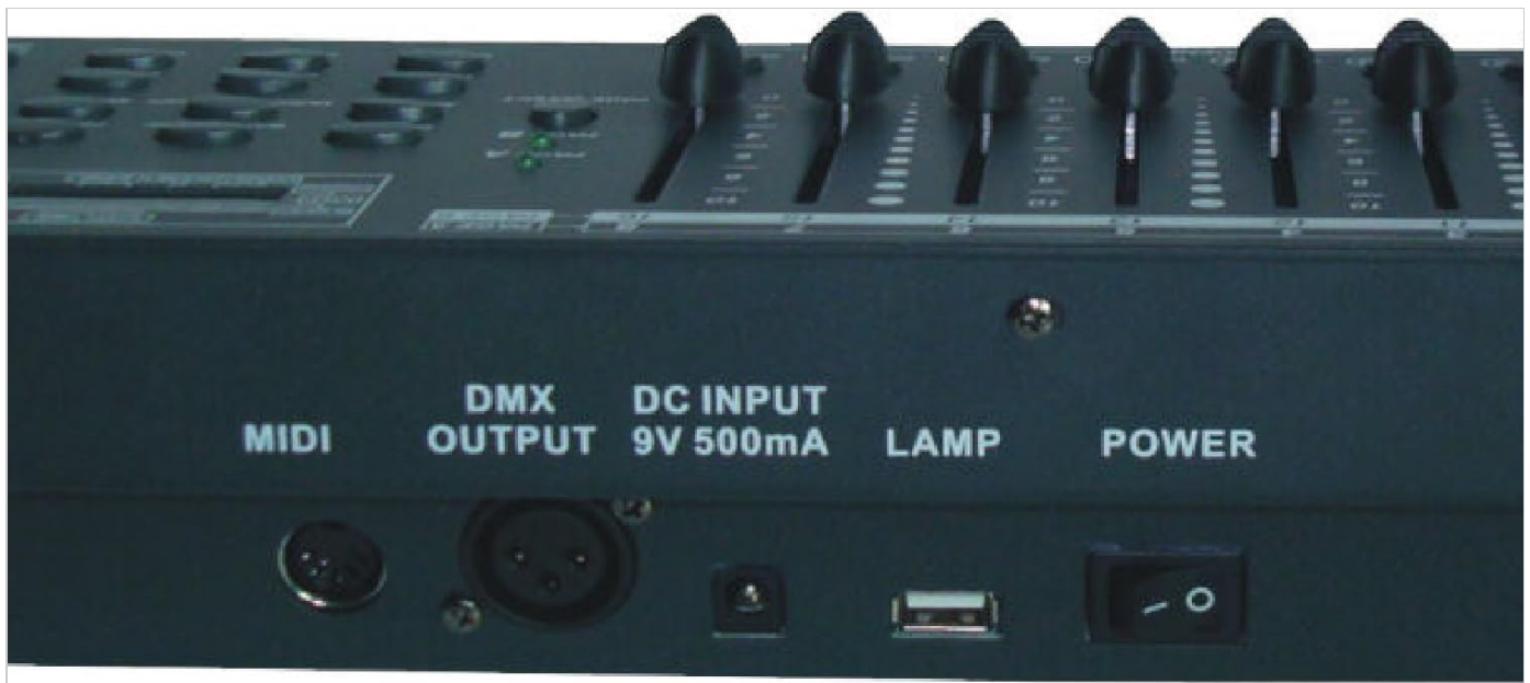
Figure 3.6: Detail of the rear panel connections, including MIDI ports, DMX output, DC power input, lamp connector, and the main power switch.
