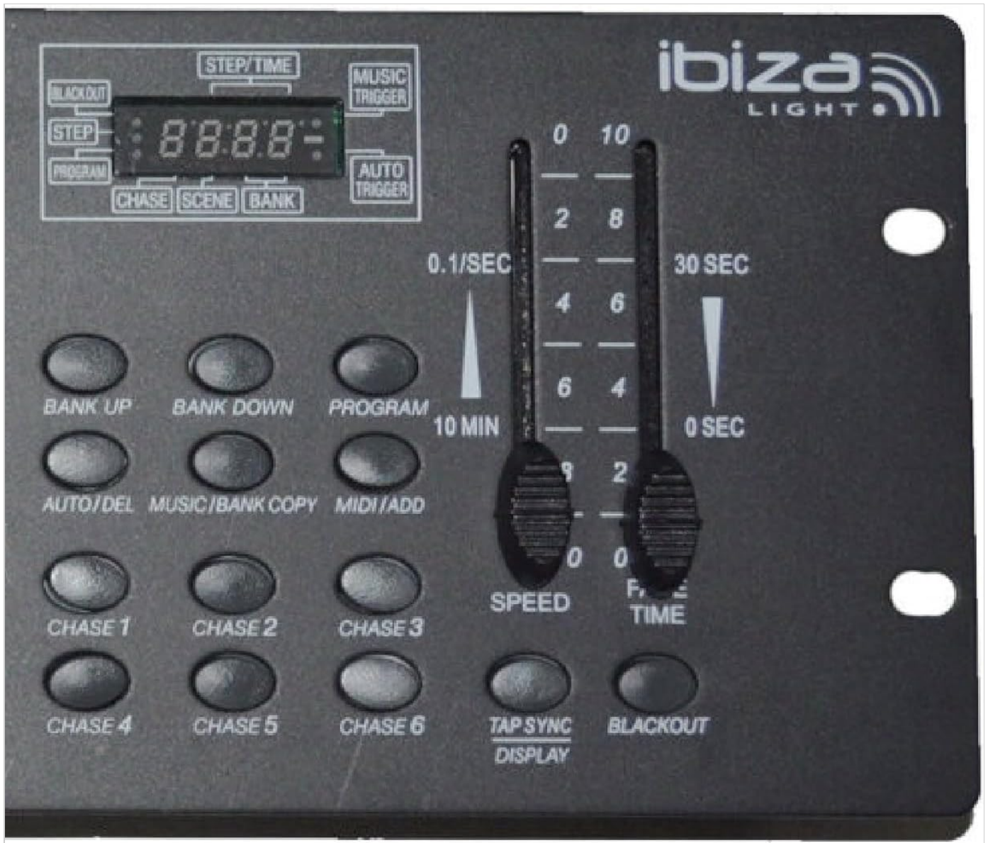
Figure 3.4: Detail of the right-hand control section, featuring the 4-digit LED display, bank navigation, program, chase selection, and faders for speed and fade time adjustments.
