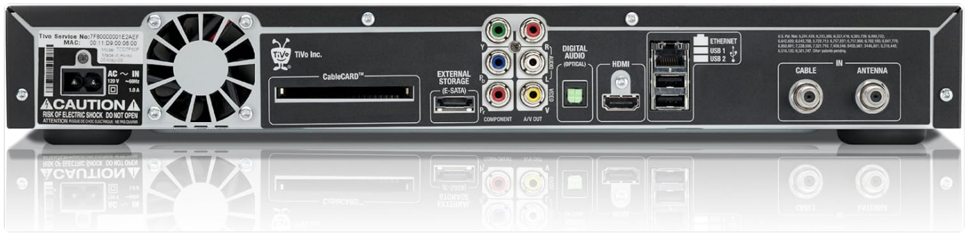
Figure 3.1: Rear panel connections of the TiVo Premiere XL DVR. This image highlights the HDMI output, Ethernet port, CableCARD slot, coaxial cable input, and other audio/video ports for connecting the device to a television and home network.
