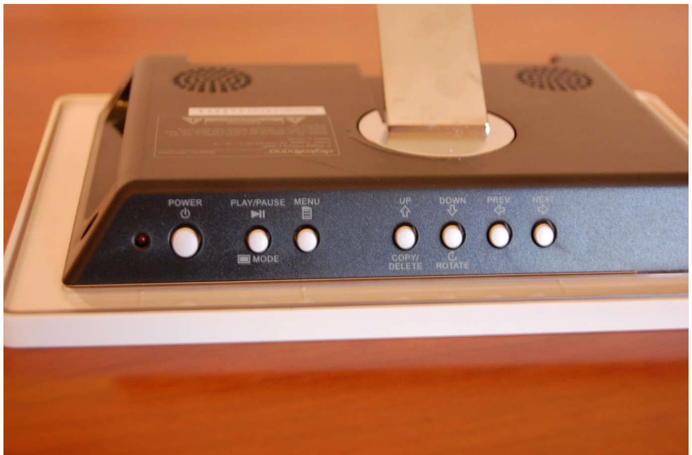
Image: Rear view of the digital picture frame, showing the control panel with buttons for Power, Play/Pause, Menu, Up, Down, Prev, Next, Copy/Delete, and Rotate.
