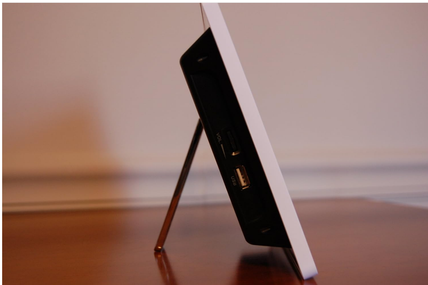
Image: Side view of the digital picture frame, showing the USB port and volume control slot.
