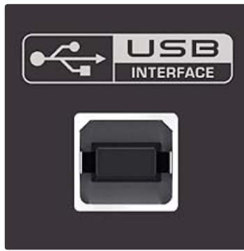
Figure 6: Depiction of the USB interface and port for computer connectivity.
