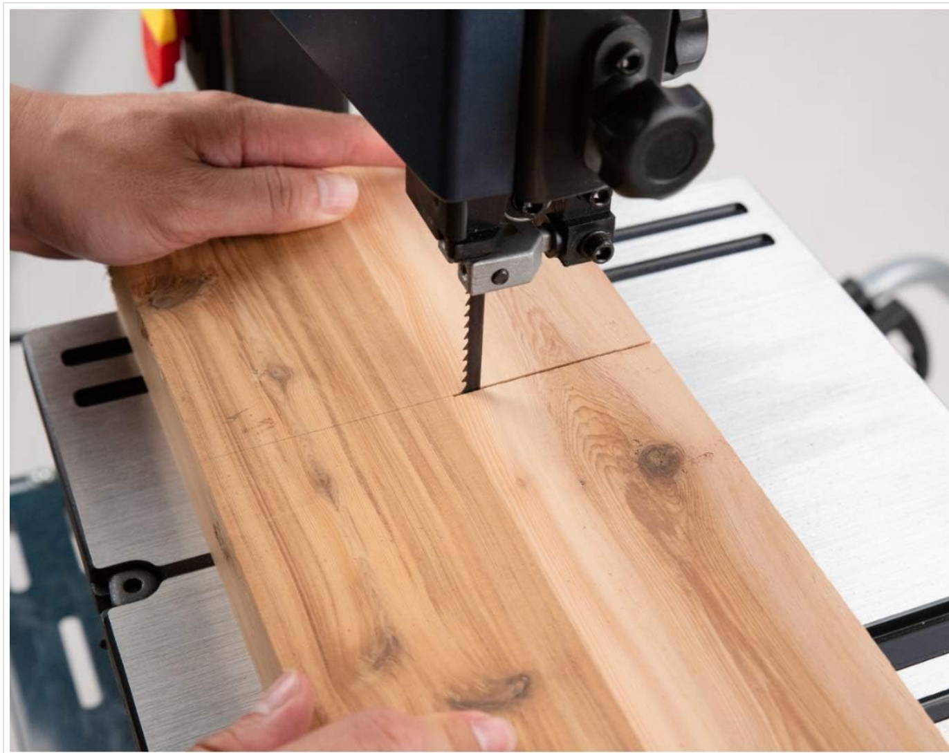
Figure 5.1.2: A user operating the POWERTEC BS900 bandsaw to cut a piece of wood, demonstrating proper hand placement and material feeding.
