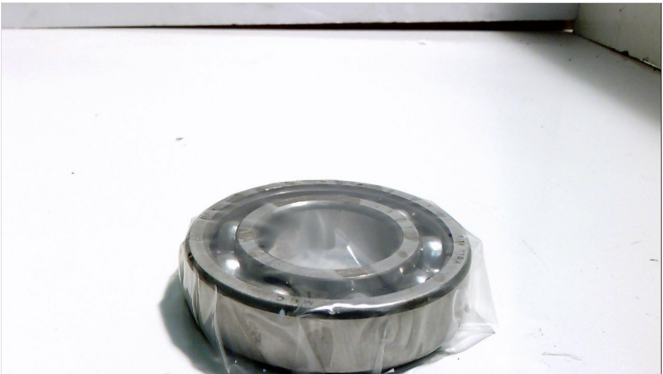
Figure 3.1: Top view of the MRC 207S bearing, showing the inner and outer rings with ball elements.
