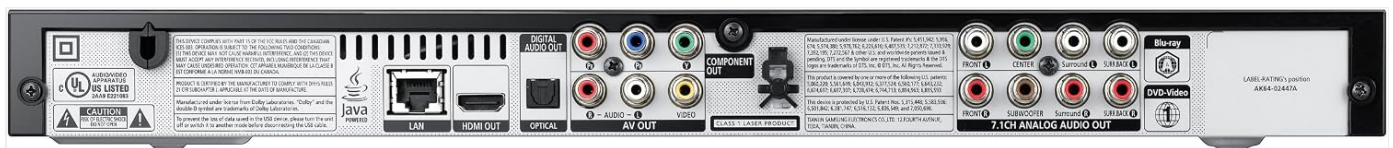
Figure 2: Rear panel connections, including HDMI, LAN, Optical, and 7.1 Channel Analog Audio outputs.
