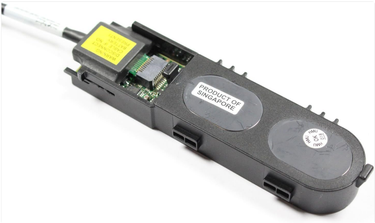
Figure 3: Bottom view of the battery module, revealing a 'PRODUCT OF SINGAPORE' label and a yellow warning label. The warning states: 'WARNING: DISCONNECT CABLE IF NO BATTERY PRESENT!', indicating a safety measure related to the module's connection within the system.
