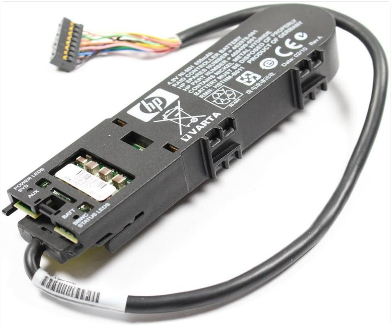
Figure 1: Top view of the HP Smart Array Battery Module, showing the main body, attached cable with multi-pin connector, and product labels. Visible labels include HP logo, VARTA logo, battery specifications (4.8V Ni-MH 650mAh), part numbers, and disposal warnings. Status LEDs for Power, System, Auxiliary, Battery, and BBWC are also indicated.
