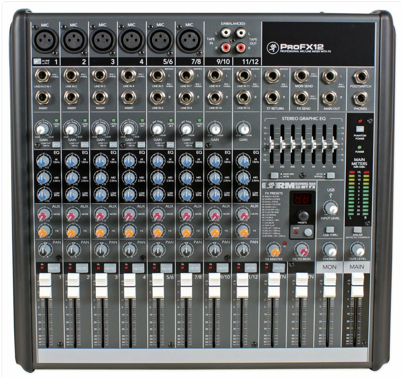
Figure 1: Mackie PROFX12 12-Channel Compact Effects Mixer. This image shows the overall layout of the mixer, including input channels, main mix section, and effects controls.
