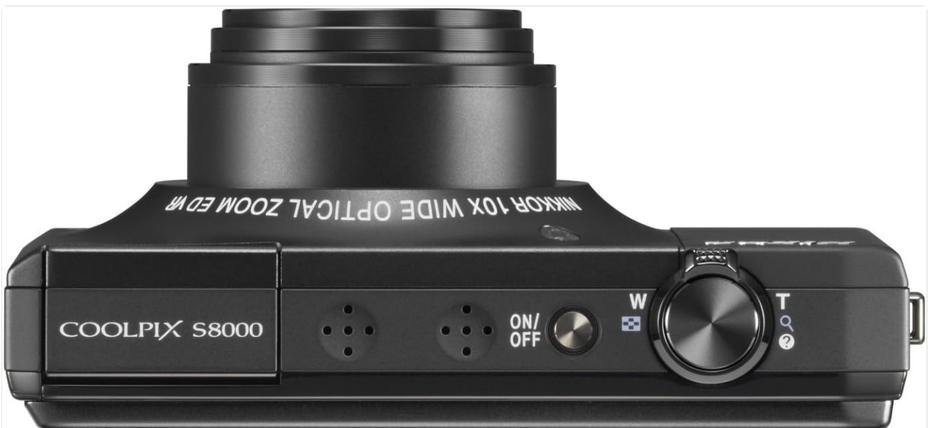
Image 3: Top view of the Nikon Coolpix S8000 digital camera. The power button, shutter button, and zoom lever are clearly visible, along with the "COOLPIX S8000" branding.
