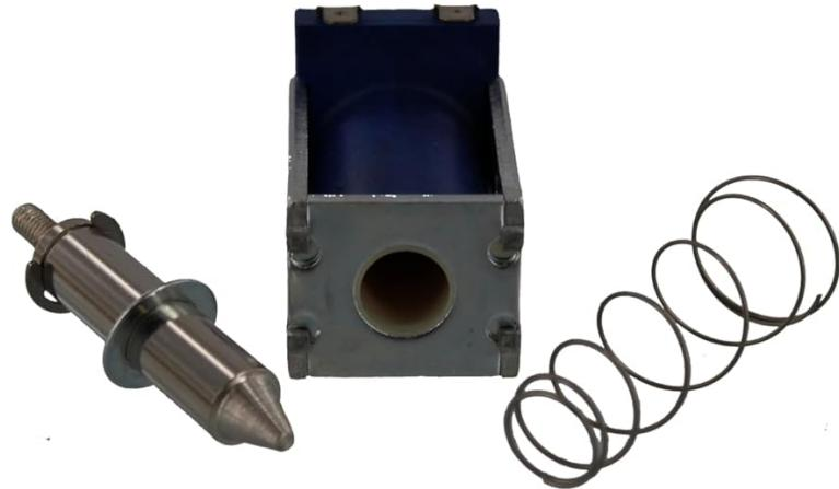
This image displays the individual components of the F300128P solenoid: the main solenoid coil housing (blue interior, grey exterior), the metallic plunger with a threaded end, and a coiled spring. These parts work together to control the door release mechanism.
