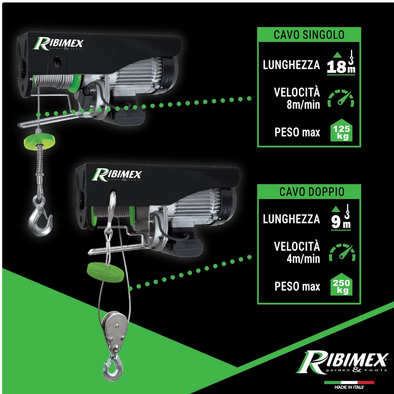
Figure 4: Single vs. Double Cable Configuration. This diagram visually explains how to set up the hoist for single-line operation (125 kg capacity, 18m height, 8m/min speed) and double-line operation using the pulley (250 kg capacity, 9m height, 4m/min speed).
