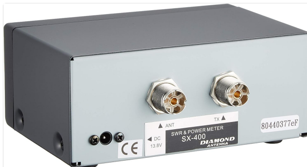
Image: Rear view of the Diamond SX400, displaying two SO-239 (UHF Female) connectors labeled 'ANT' for antenna and 'TX' for transceiver, along with the 13.8V DC input for the backlight.
