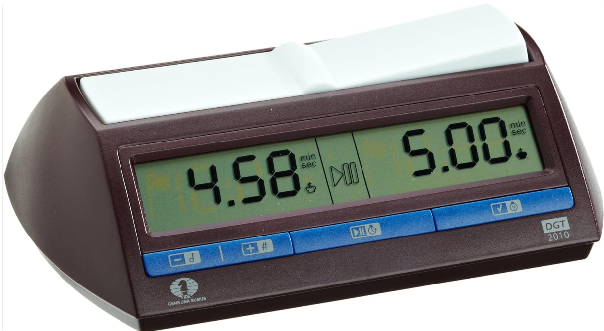
Figure 1: Front view of the DGT DGT2010 Digital Chess Clock. The display shows time for two players, and the blue buttons are visible at the bottom.
