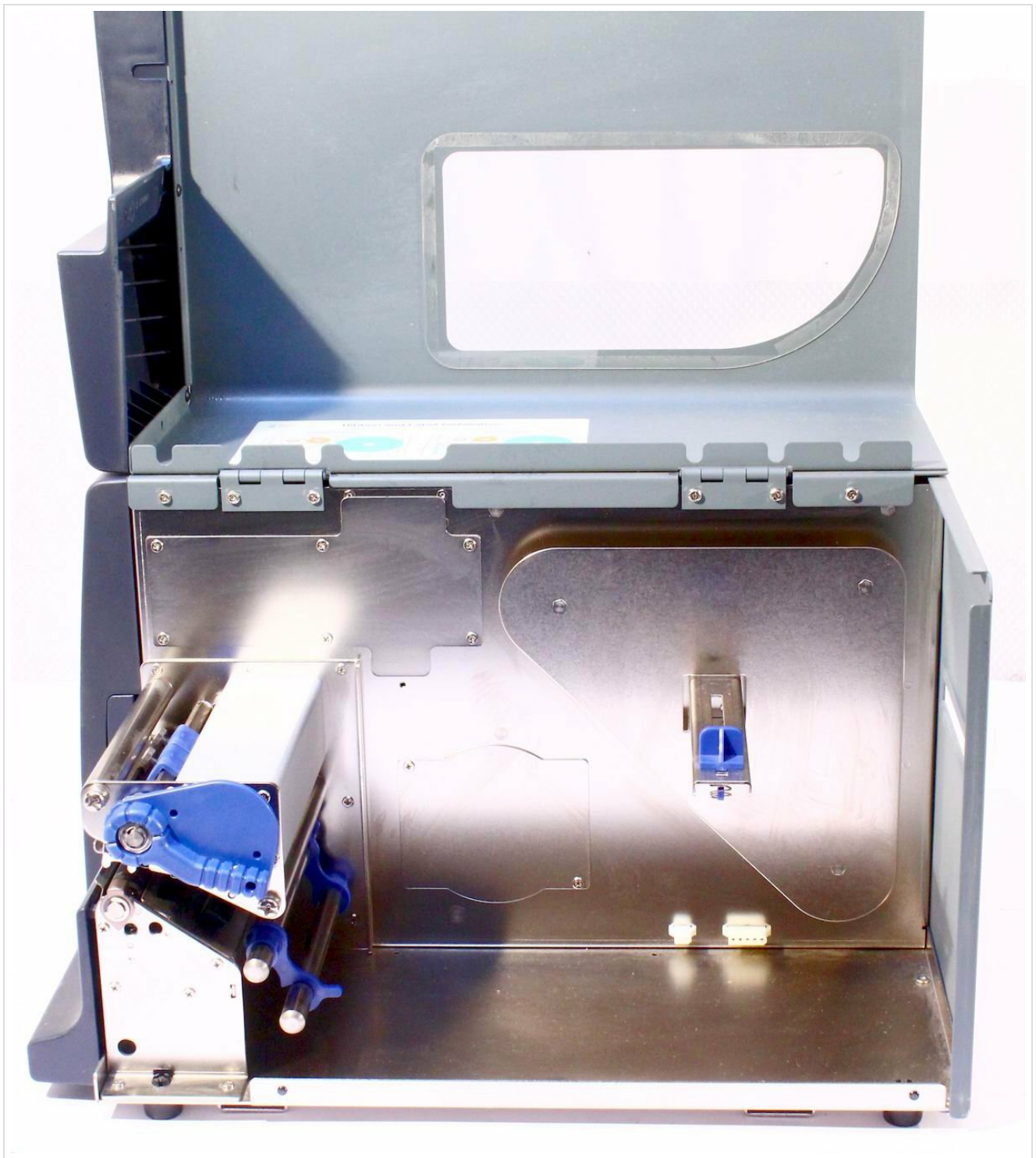
Figure 4.3: Internal View of the Intermec PD42 Printer. With the top cover open, this image reveals the internal mechanisms for loading labels and ribbon. Key components such as the printhead assembly, media guides, and ribbon spindles are visible, illustrating the media path.
