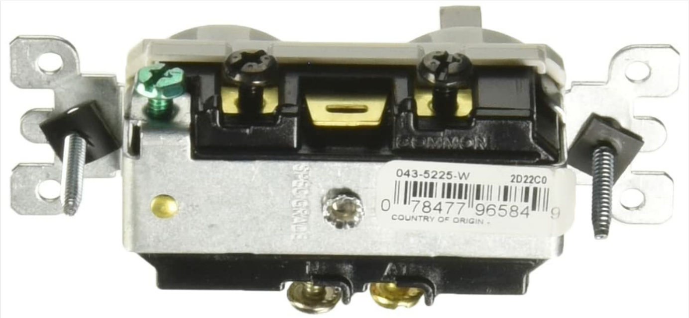
Figure 2: Back view of the Leviton 5225, illustrating the brass (hot), silver (neutral), and green (ground) wiring terminals, along with the break-off tab. The UPC 0078477965849 is visible.
