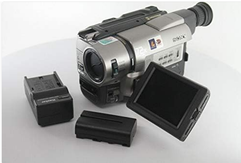
Image: The Sony CCD-TRV85 camcorder displayed with its 3.5-inch LCD monitor open, alongside a removable battery pack and a battery charger. This illustrates the main components for initial setup.
