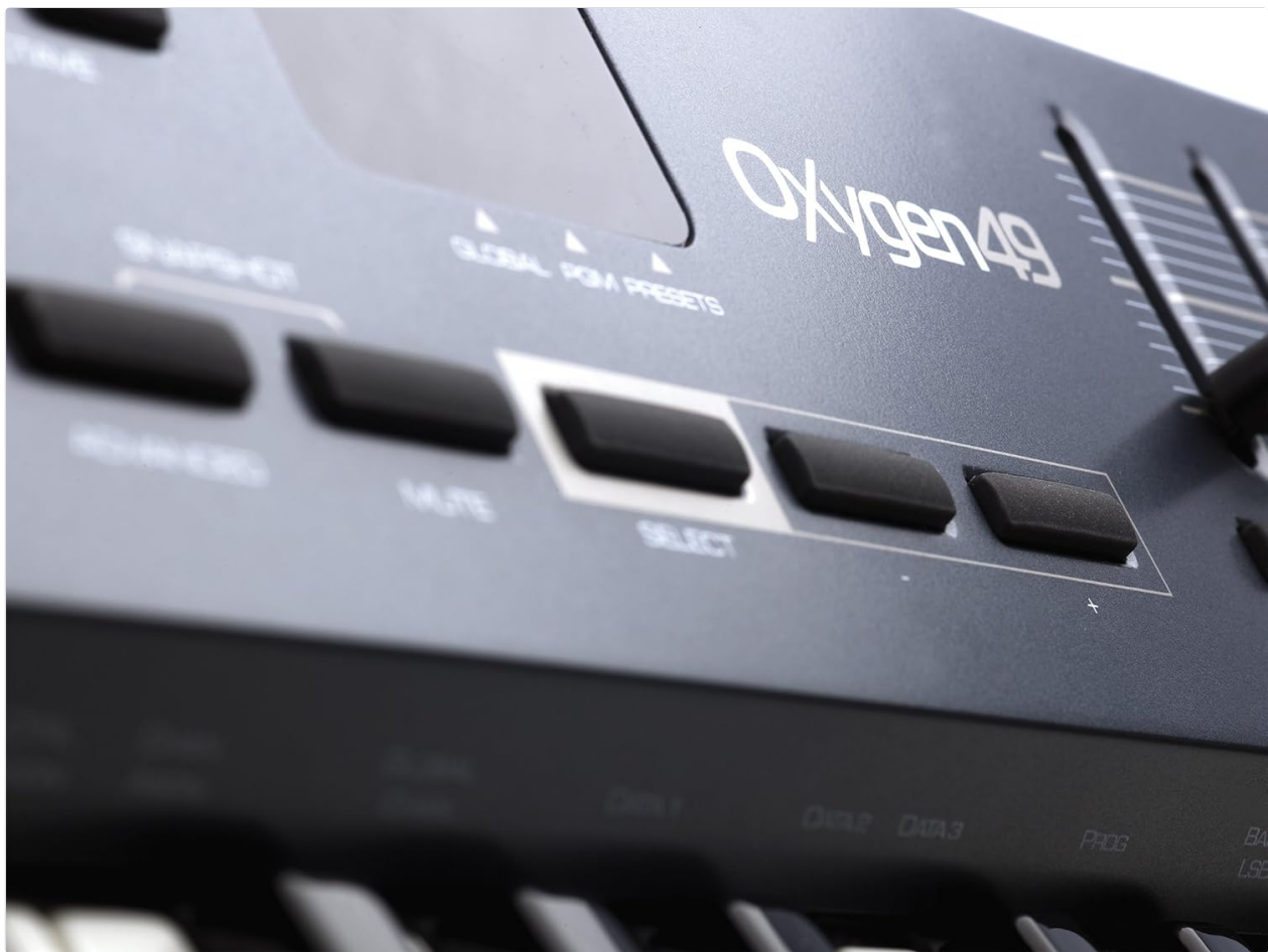
Figure 3: Detailed view of the transport controls and other assignable buttons on the Oxygen 49 MK III, including 'Select' and 'Global' functions.
