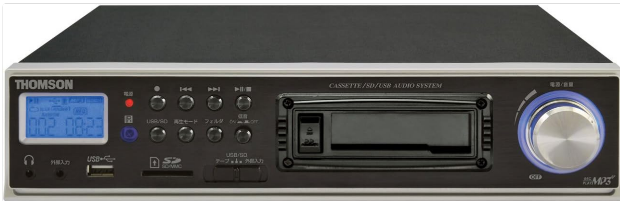
Figure 2.1: Front Panel View. This image displays the front of the THOMSON CE-26 unit, showing the cassette deck, control buttons, display screen, USB port, SD/MMC card slot, and volume knob.
