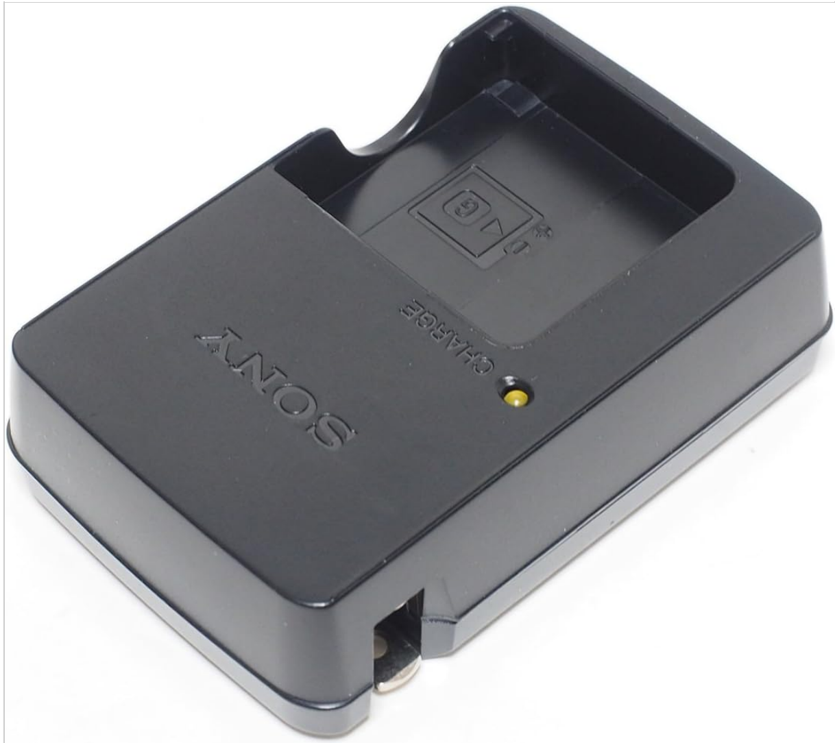
Figure 5.1: The Sony BC-CSG charger with a battery inserted, showing the location of the yellow charge indicator LED.
