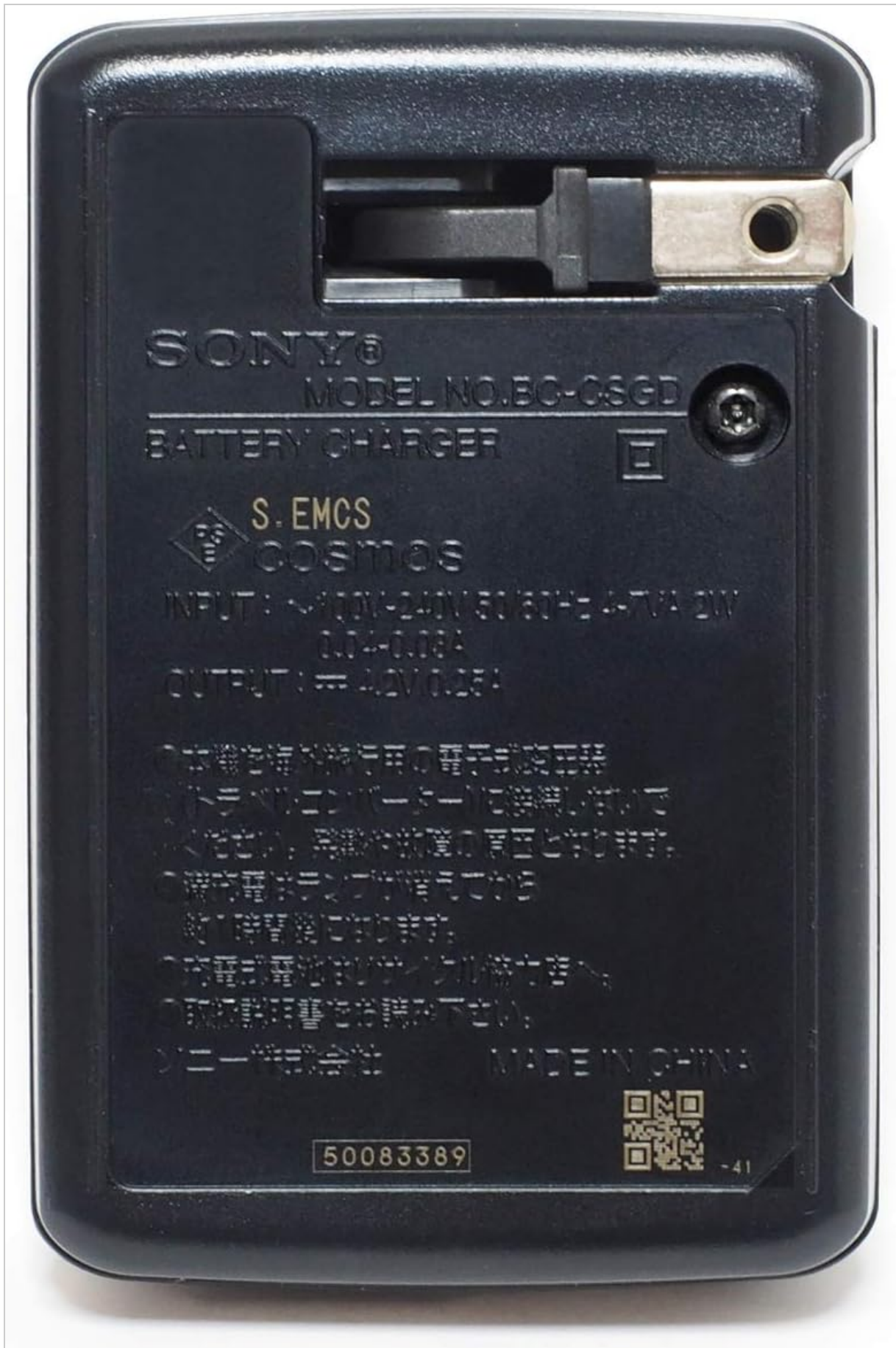
Figure 4.2: Back view of the Sony BC-CSG charger, illustrating the foldable AC power prongs for direct wall connection.
