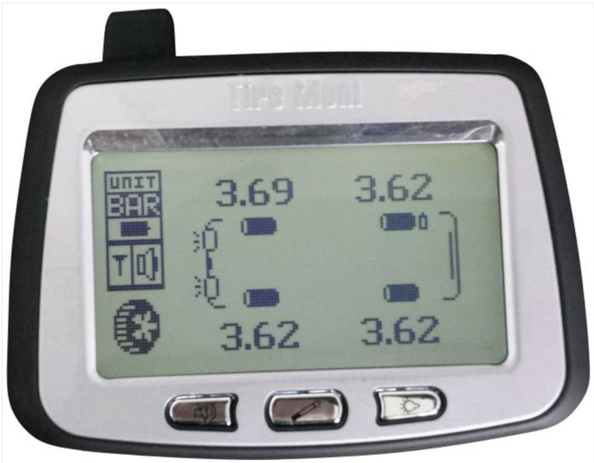
Image 2.1: TireMoni TM-240 Display Unit and Sensors. This image shows the main display unit and the four external tire pressure sensors included with the system.
