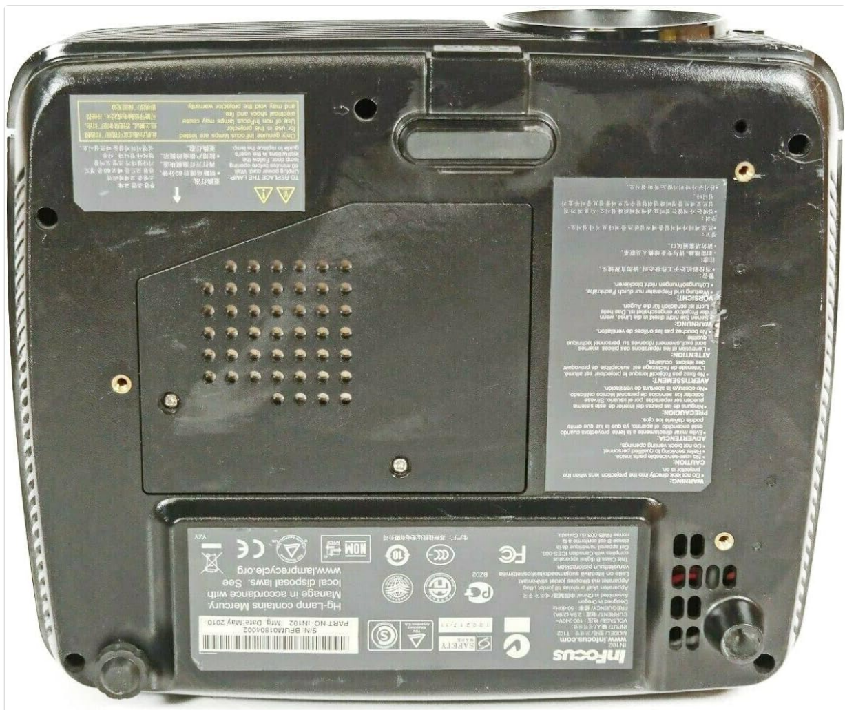
Figure 3.4: Bottom View of the IN102 Projector. This image displays the underside, revealing the mounting points for ceiling installation and the adjustable feet for leveling.
