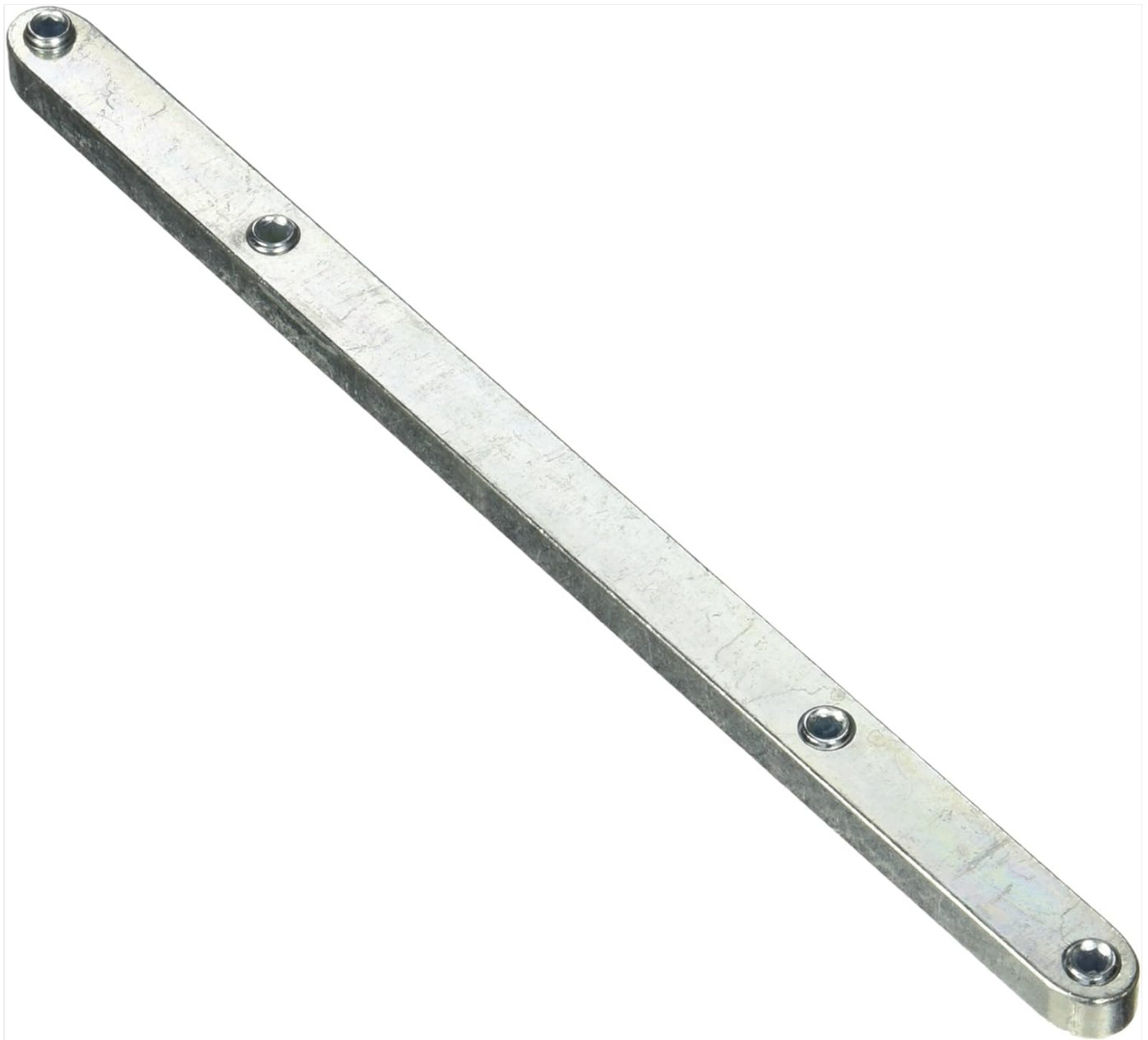
Image 1.1: The Festool 484455 Connection Bar, a steel bar with four integrated pressure screws for joining MFT tables.
