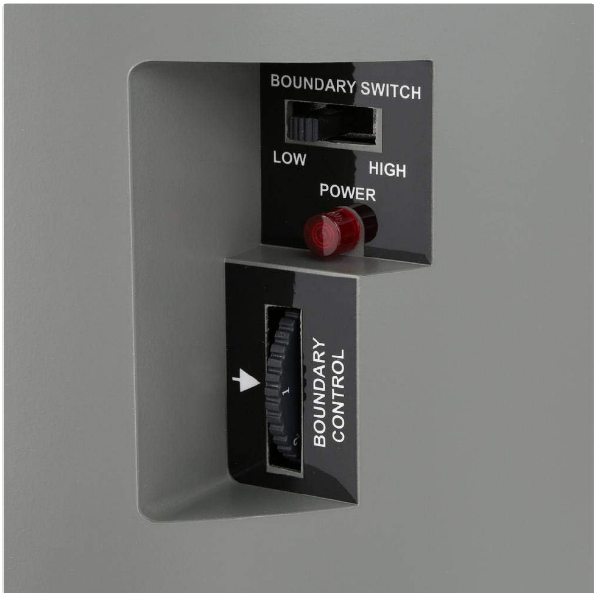
Image 4.2: Close-up of the PetSafe Wireless Transmitter, highlighting the Boundary Switch (LOW/HIGH) and Boundary Control dial.
