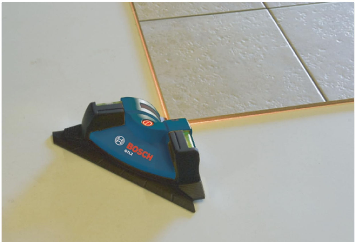
Figure 3: The BOSCH GTL2 projecting laser lines on a tiled floor, demonstrating its utility for precise tile layout.
