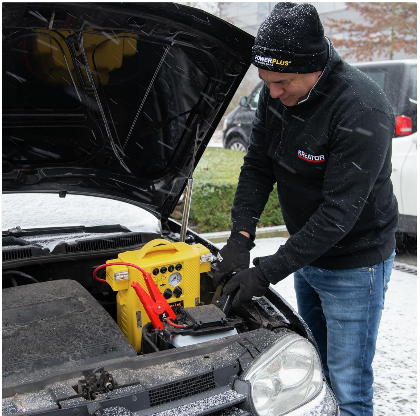
Figure 3: Using the Power Station to jump start a vehicle.
