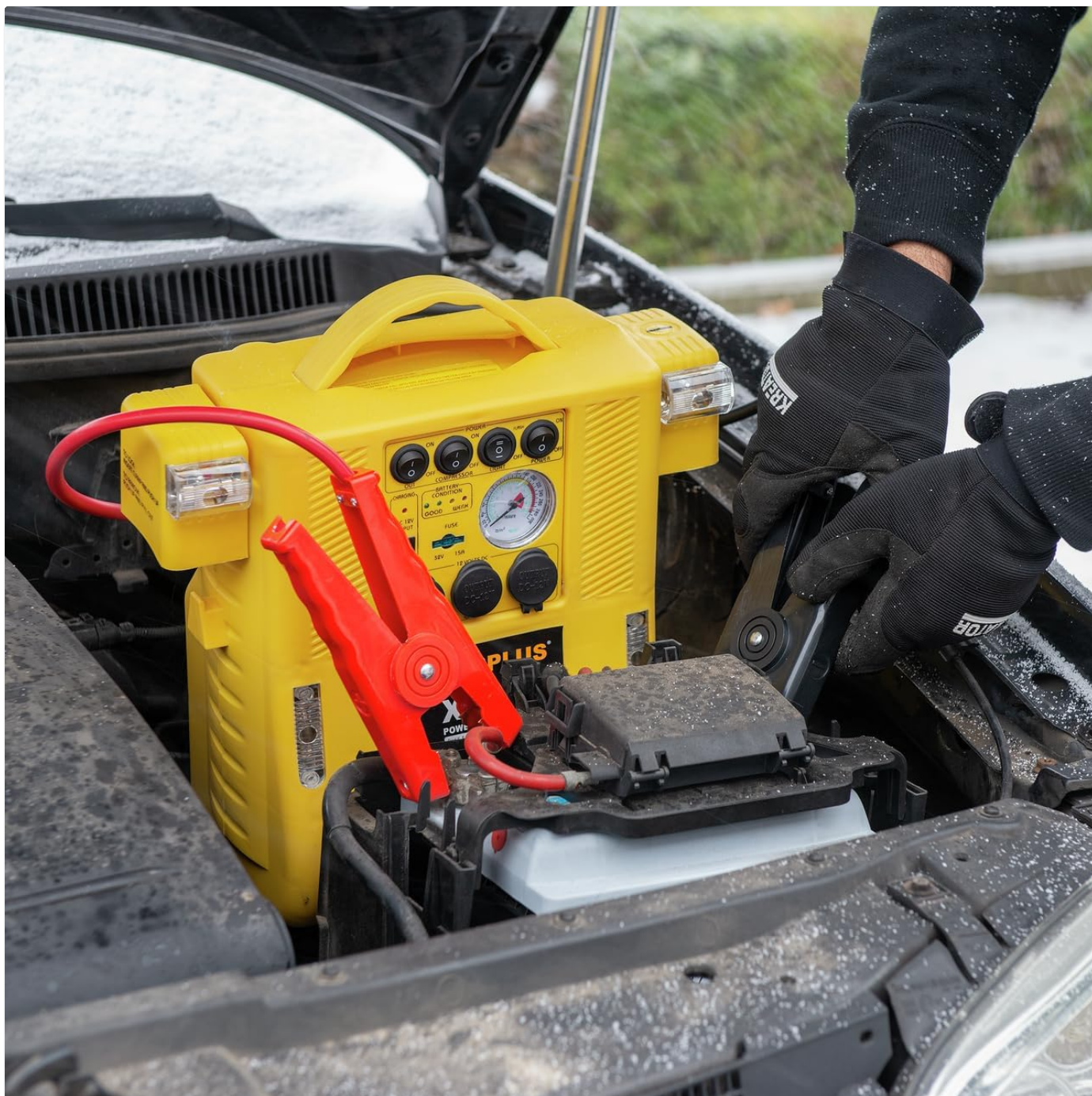
Figure 4: Proper connection of jumper clamps to battery terminals.
