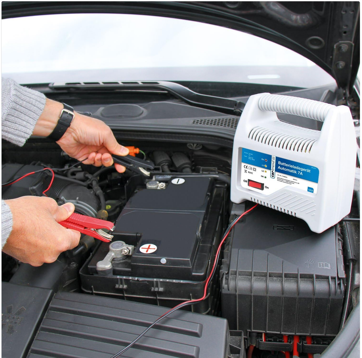
Figure 2: Illustrates the connection of the battery charger clamps to a car battery. The red clamp is attached to the positive terminal and the black clamp to the negative terminal, with the charger unit placed securely nearby.
