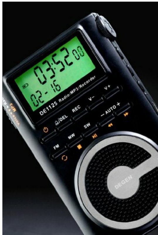
Figure 3.1: Close-up view of the DEGEN DE1125's display and control panel, showing buttons for power, mode selection, tuning, and volume.
