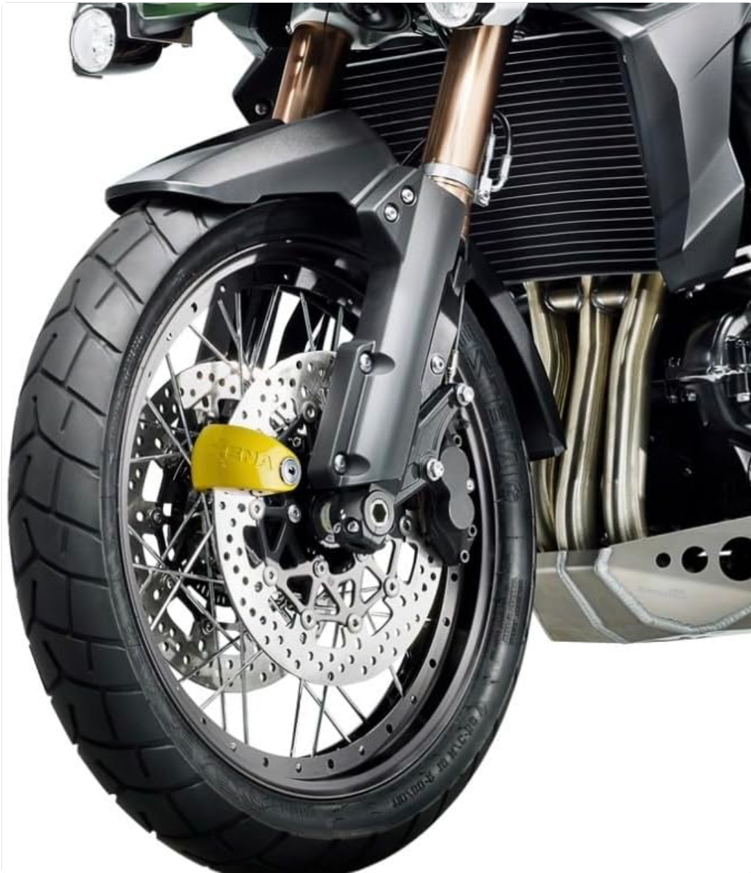
Figure 3: The XENA XX6 disc lock alarm securely installed on the front brake disc of a motorcycle, demonstrating its compact fit.
