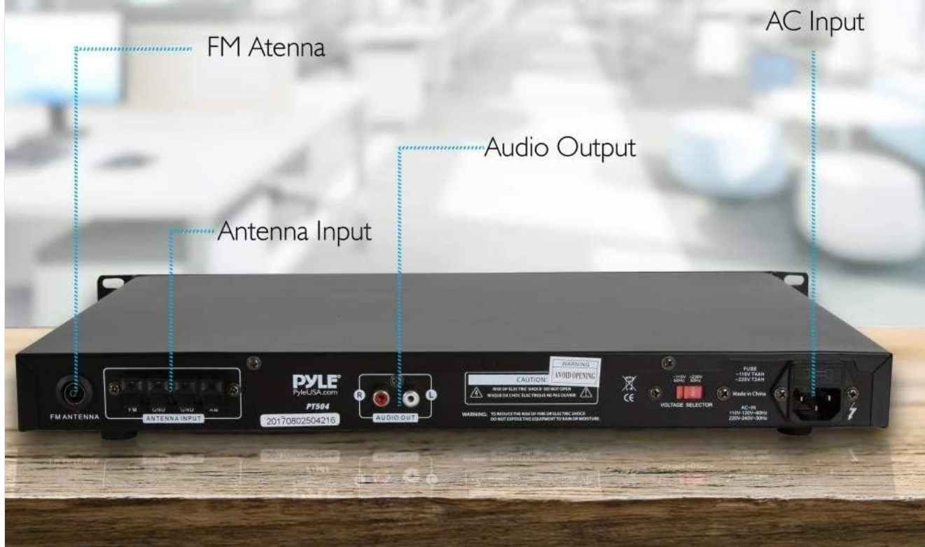
Figure 4.2: Rear panel of the PyleHome PT504 digital AM/FM tuner, showing input and output connections. From left to right, it includes an FM antenna input, AM antenna input, audio output (RCA L/R), and an AC power input with a 110V/220V voltage selector switch. Labels clearly indicate each port's function, essential for proper setup and connectivity.
