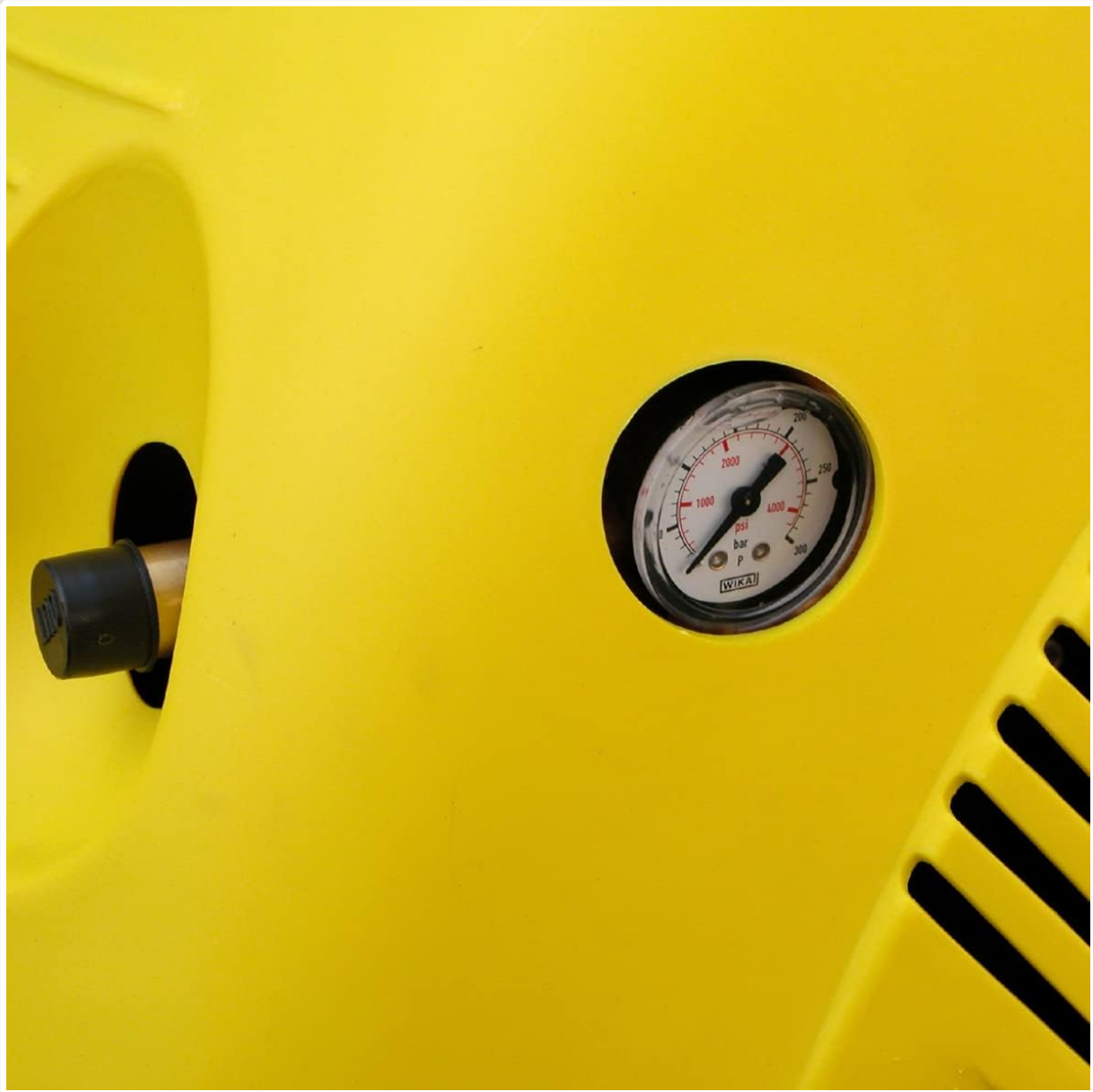
Image 3.2: Pressure Gauge. This image highlights the pressure gauge, indicating the operational pressure in bar and PSI.
