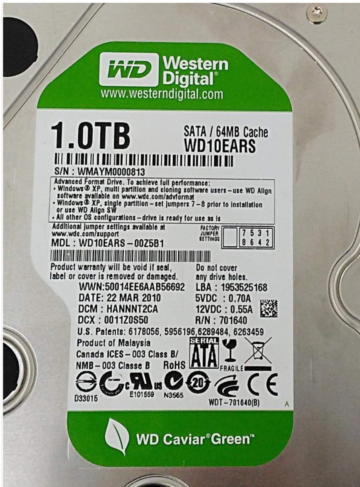
Figure 2: Close-up view of the product label on the Western Digital Caviar Green WD10EARS hard drive. The label displays key information including the serial number (S/N: WMAYM0000813), model number (MDL: WD10EARS-00Z5B1), manufacturing date (DATE: 22 MAR 2010), and electrical specifications (5VDC: 0.70A, 12VDC: 0.55A). It also notes the requirement for the WD Align utility for Windows XP due to Advanced Format (AF) technology.
