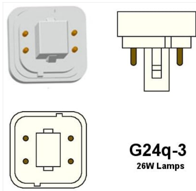
Figure 2: G24Q-3 Base Diagram. This diagram illustrates the pin configuration of the G24Q-3 base, essential for proper alignment during installation.
