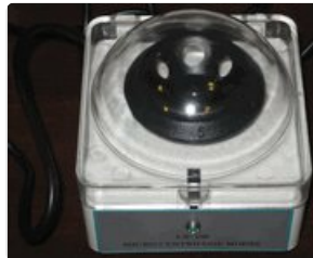
Figure 1: The CB Mini Microcentrifuge unit. This image shows the compact Mini Microcentrifuge unit. It features a white base with a clear, hinged lid, revealing the black rotor inside. A power cord extends from the back of the unit.
