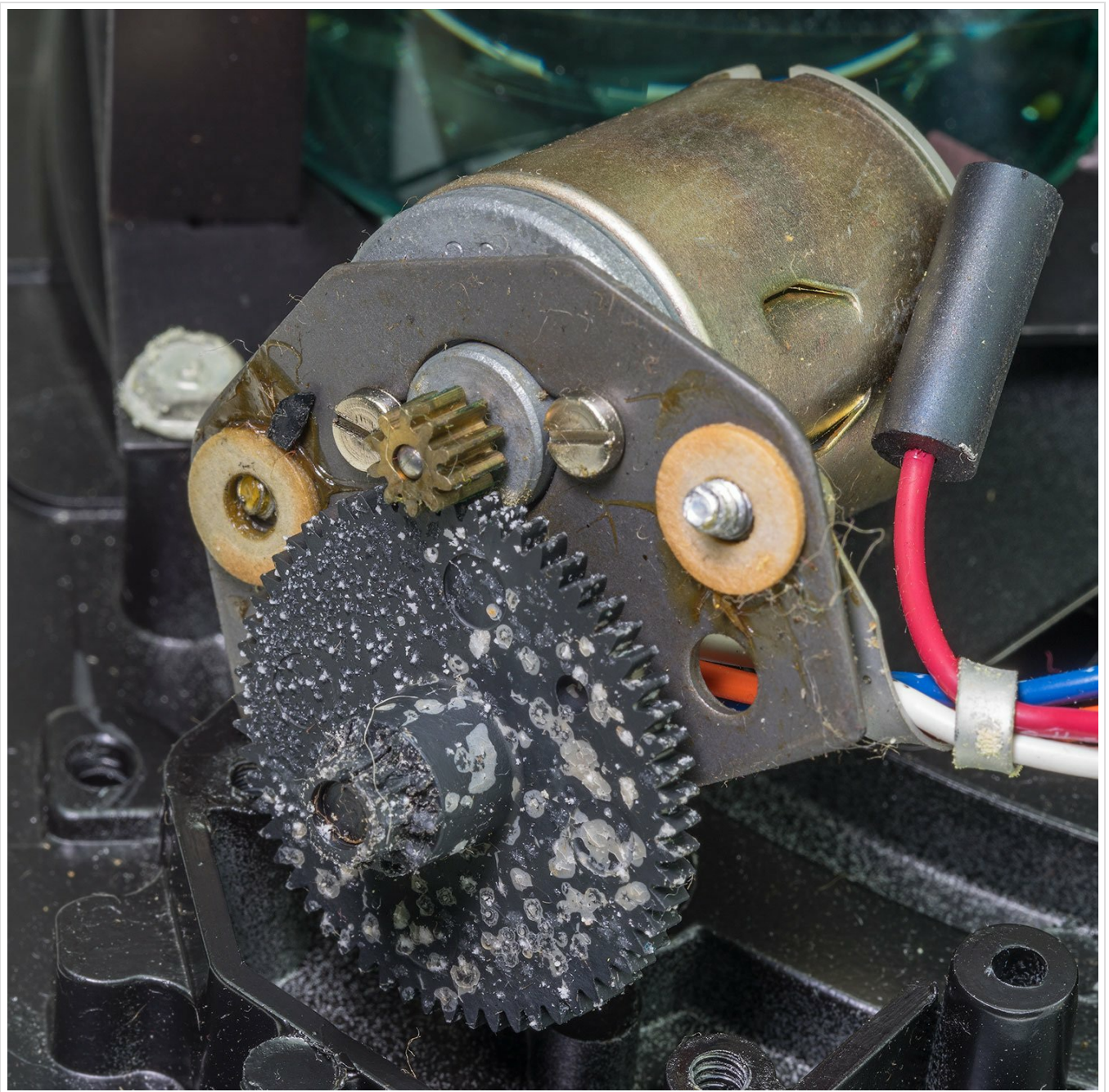
Figure 2: An example of a worn main drive gear inside a Bell & Howell Cube Slide Projector. Note the visible damage and debris around the gear, indicating wear that prevents proper slide advancement.
