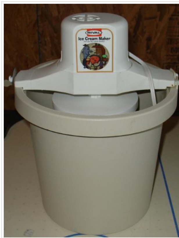
Figure 1: Overview of the Rival Ice Cream Maker Model 8401. This image displays the assembled unit, including the motor unit, lid, and outer bucket, with the inner plastic jug visible.
