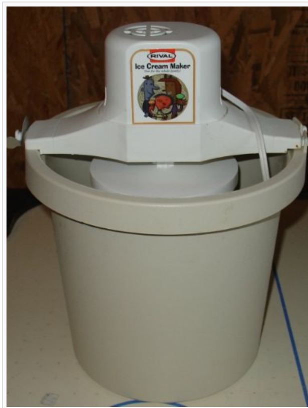
Figure 2: The Rival Ice Cream Maker Model 8401 fully assembled and ready for the churning process. Note the motor unit securely placed on the outer bucket, with ice and salt surrounding the inner jug.
