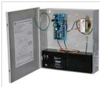
Figure 1: Altronix AL175X220 Power Supply with enclosure open.
