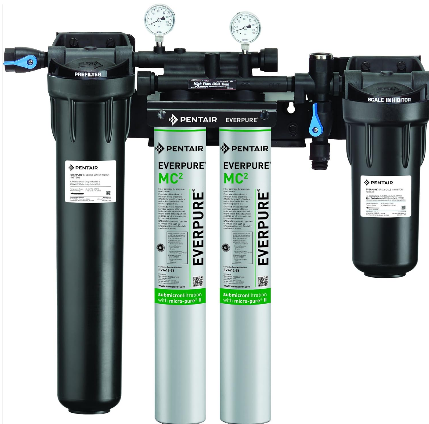
Figure 1: Everpure EV933042 High Flow CSR Twin-MC2 System. This image displays the complete water filtration system, including the prefilter housing on the left, two Everpure MC2 filter cartridges in the center, and a scale inhibitor feeder on the right. Pressure gauges are visible at the top, indicating system pressure.
