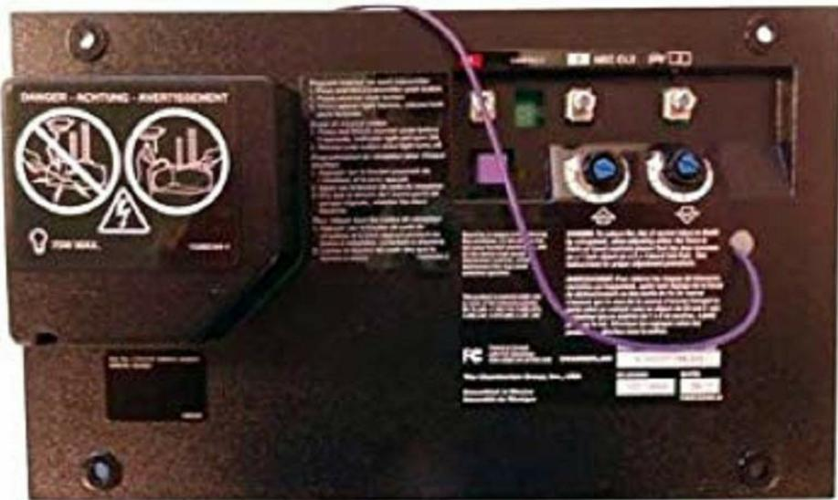
Figure 1: LiftMaster Chamberlain 41A5021-1H-315 Garage Door Opener Circuit Board. This image displays the main circuit board with various connectors and electronic components.
