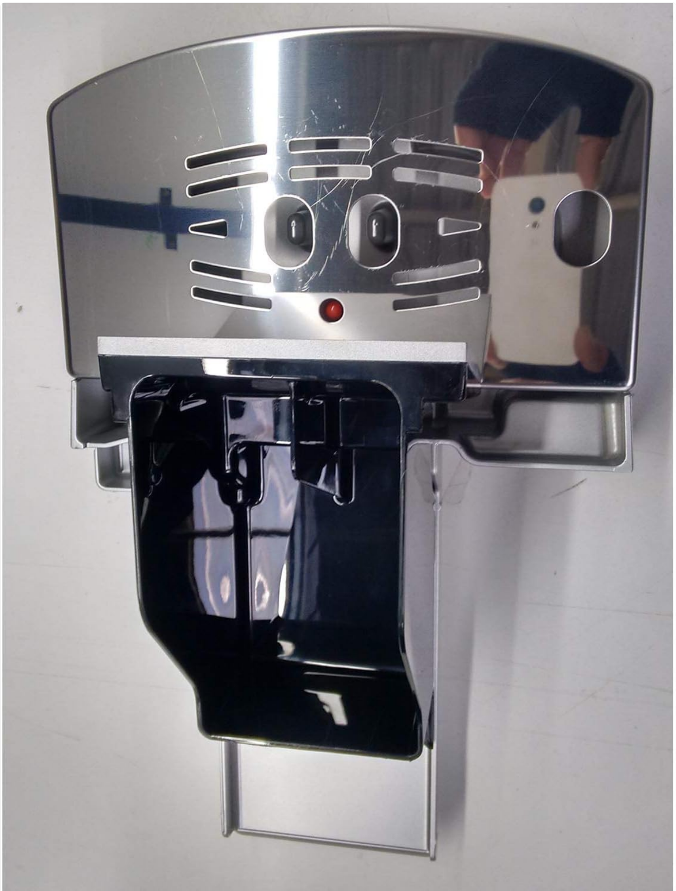
Figure 6: The removable brewing unit, essential for regular cleaning to maintain coffee quality.
