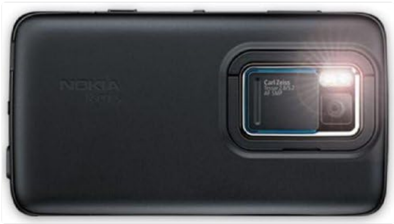
Image: Rear view of the Nokia N900, highlighting the 5-megapixel Carl Zeiss optics camera with its lens cover and dual LED flash.
