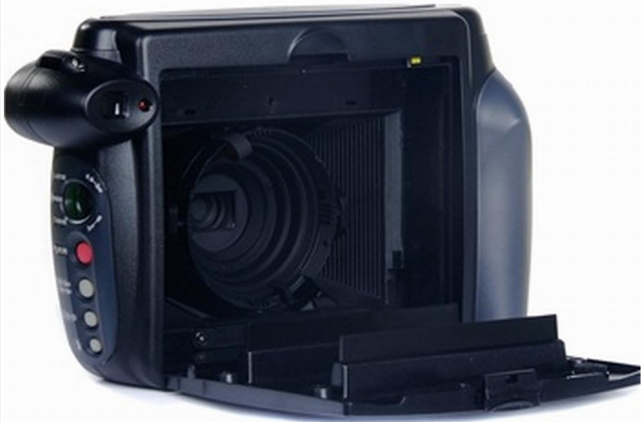
Figure 5.2: Film Compartment Area for loading Instax Wide film packs.
