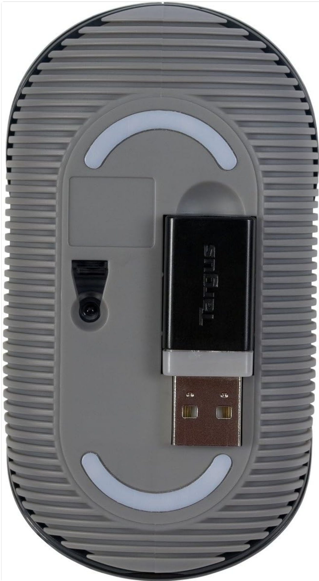
Image 4: The underside of the Targus Wireless Mouse, showing the storage compartment for the Micro USB receiver.
