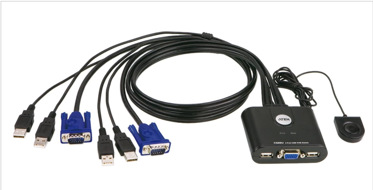
Image 2.1: The ATEN CS22U KVM switch, showing the main unit, integrated KVM cables (VGA and USB), and the remote port selector button.
