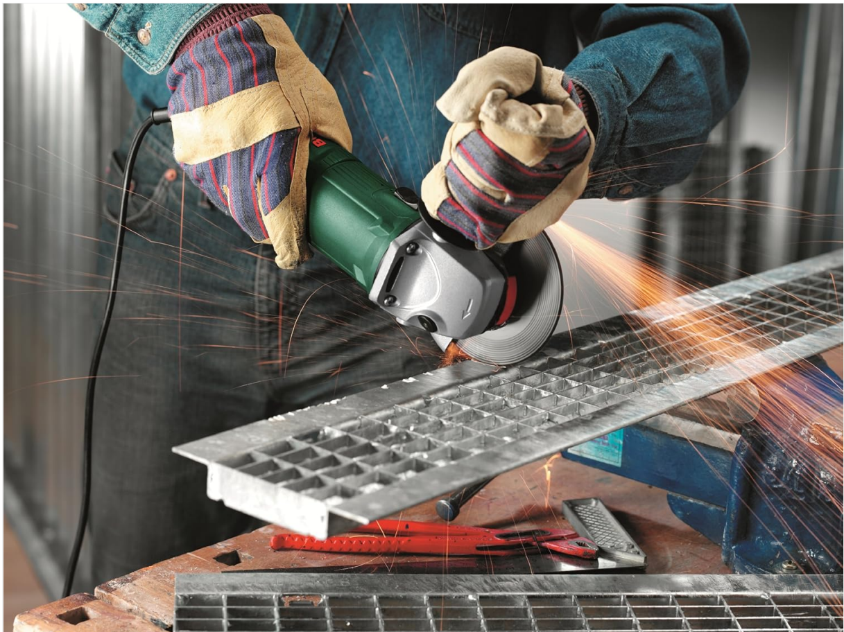
Image 2: Grinding a metal grate with the PWS 600, illustrating the sparks generated during operation.
