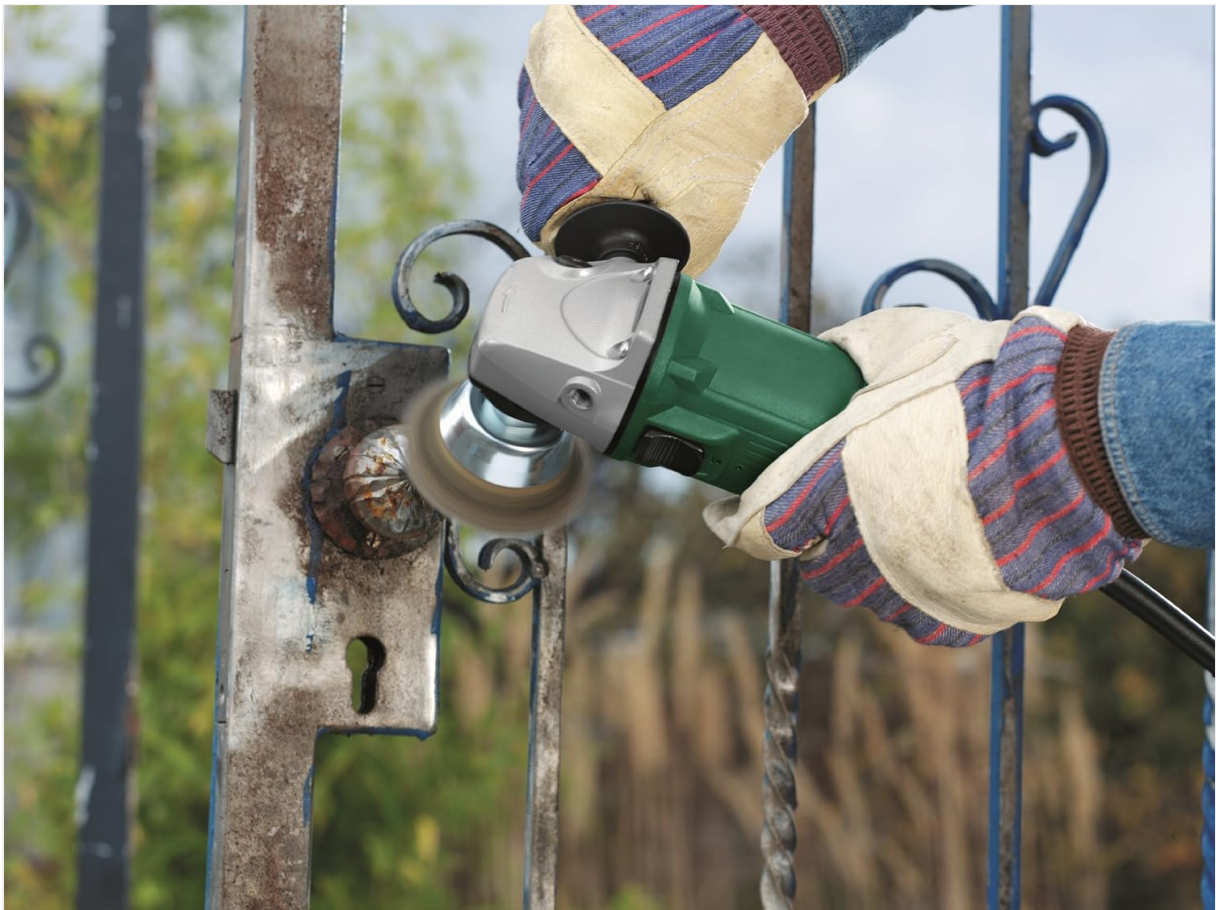
Image 4: Using the PWS 600 with a wire brush to remove rust from a metal gate, showcasing its versatility.
