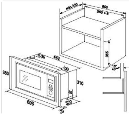
This diagram illustrates the required cabinet dimensions for installing the Amica EMW 13190 E microwave. It shows the microwave's external dimensions and the cutout dimensions for the built-in cavity, including width, height, and depth measurements in millimeters.
