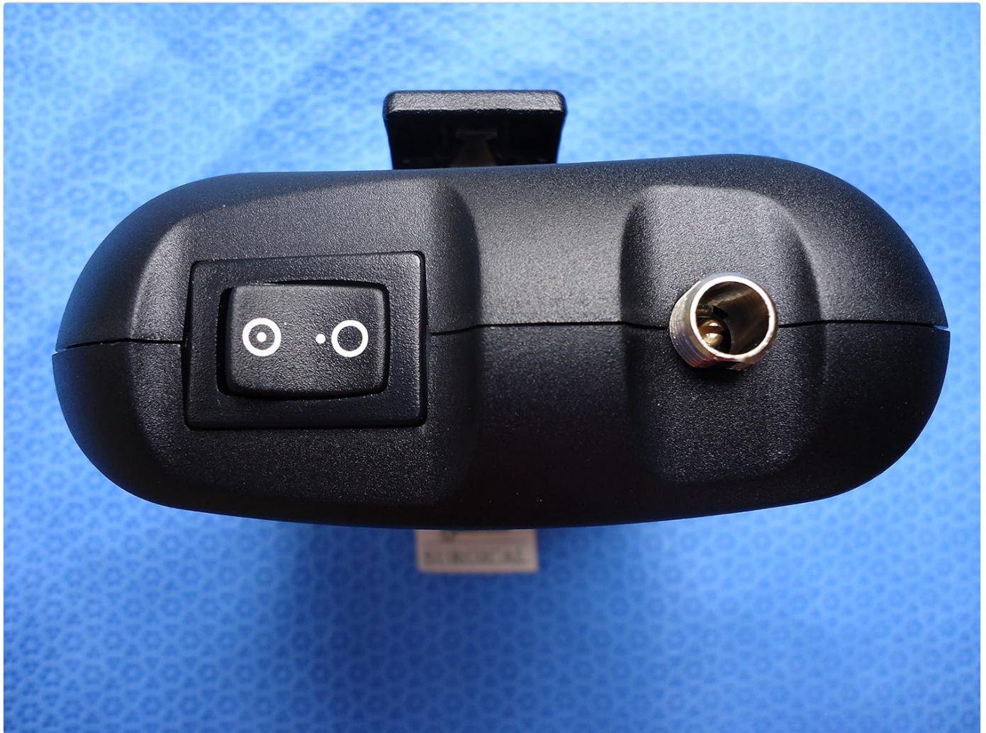
Figure 1: Top view of the battery pack, illustrating the power switch and the output port for connecting to a LumiView device.
