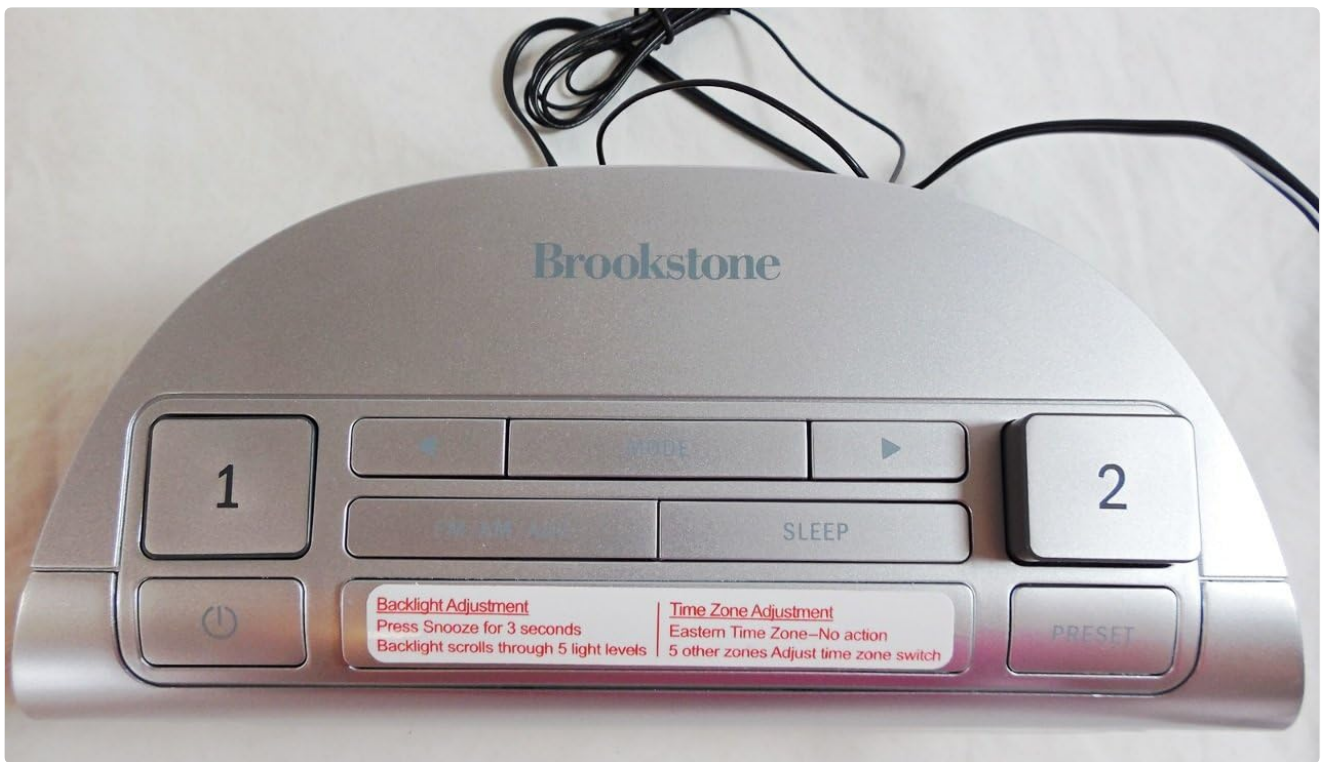
Image 3: Top view of the alarm clock, highlighting the control buttons including Alarm 1, Alarm 2, Mode, Sleep, and Preset buttons. Labels for Backlight Adjustment and Time Zone Adjustment are visible.
