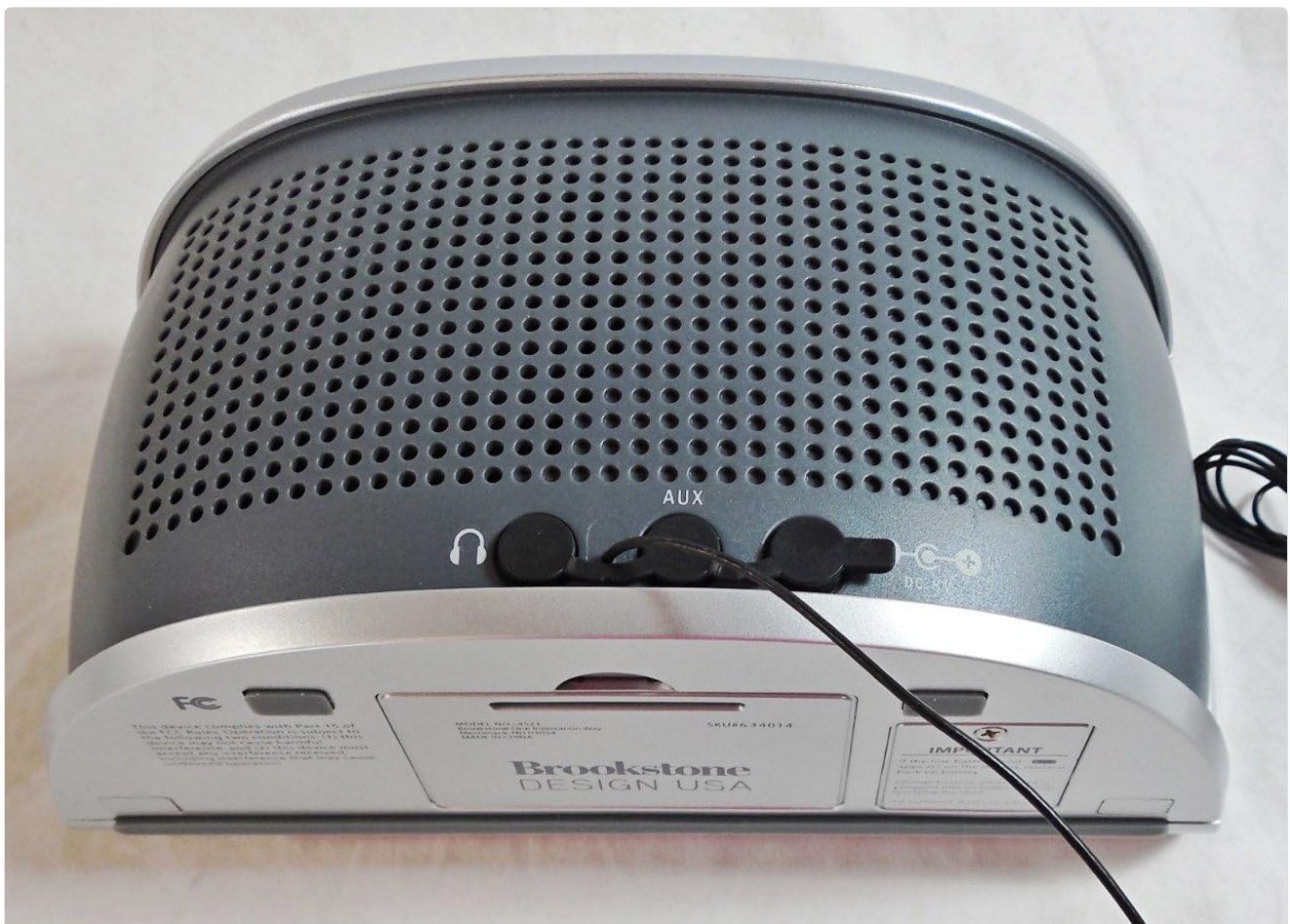
Image 4: Rear view of the alarm clock, showing the speaker grille, AUX input, and power input port. FCC compliance information and model number are also visible.
